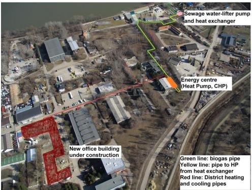
The completed heating and cooling system went for a trial run with successful results. The control system software programming has been done. All the planned elements of the system will be fully monitored and controlled by the energy controlling system.
